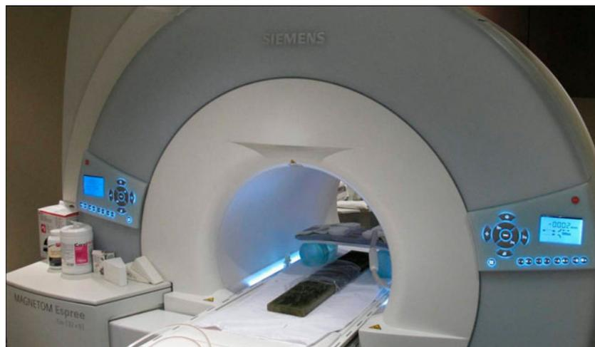
Figure 4. MRI system used for imaging the presence of water in the WPC boards.
