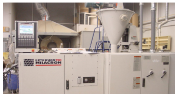
Figure 5. Cincinnati Millicon twin screw extruder used for extrusion
