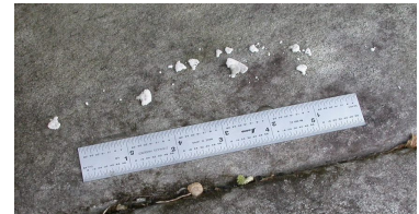
Figure 4. Decay fungi growth on wood plastic composite made without the addition of zinc borate.
