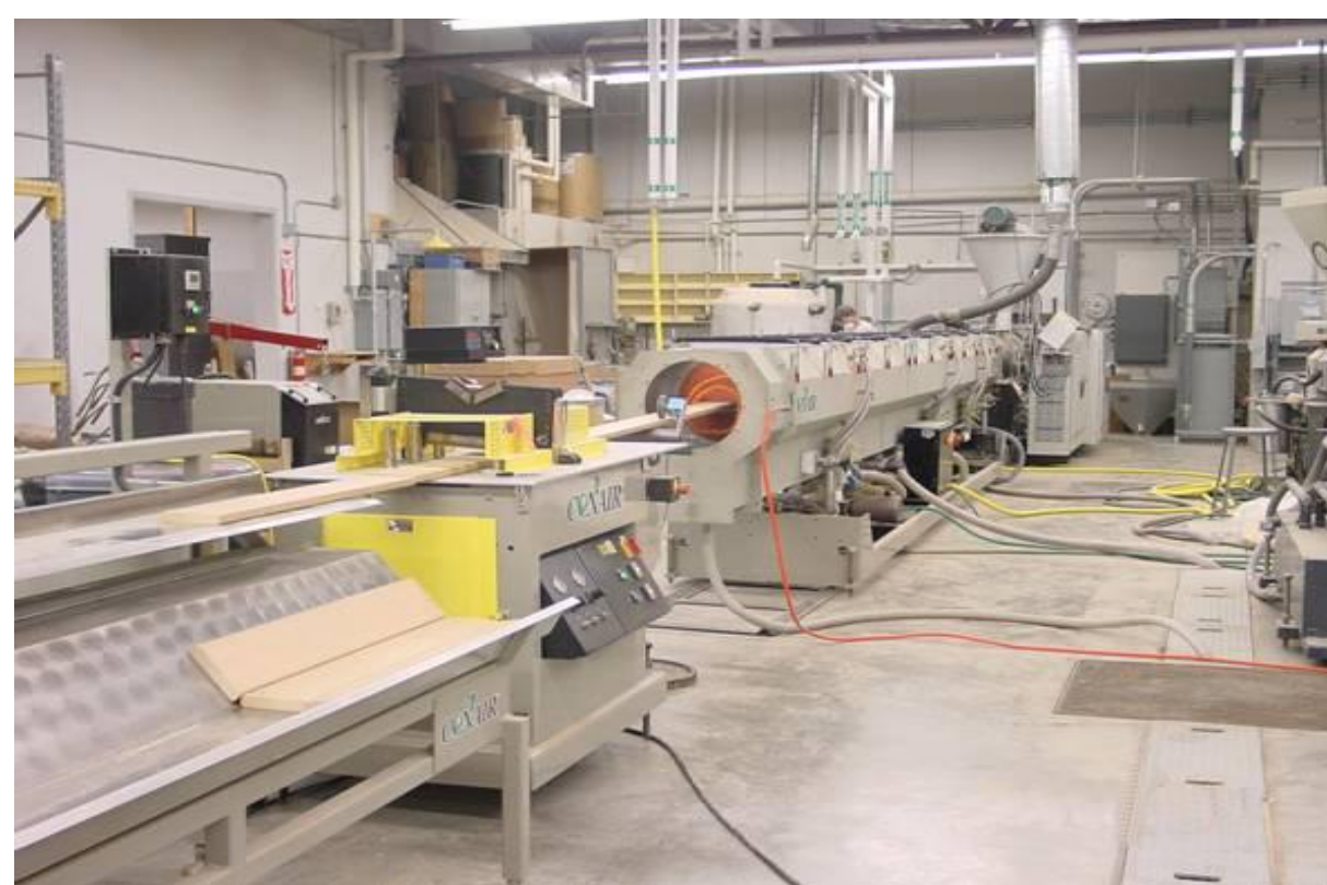
Figure 1. Manufacturing of experimental WPC boards at WSU Wood Materials and Engineering Lab
