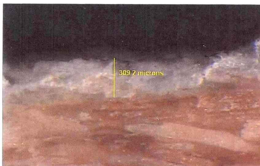
Figure 21. Depth of UV degradation after 2000 hours QUV as seen under optical microscopy
