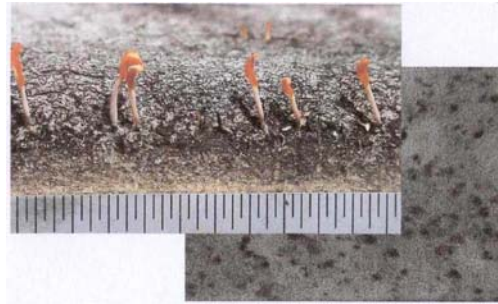
Figure 5. Acceleration of microbiological activity due to ultraviolet radiation
